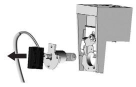
**13.** Carefully unplug the halogen lamp from the plug panel.
